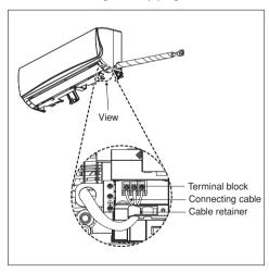
2. Secure the cable onto the control board with the cable retainer.
